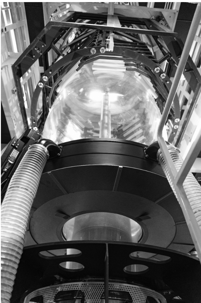
Height Adjustable Automatic Air-Ring for Stretch Hood Film running on a Die Ø of 300mm with an output of 350 – 400kg/hr
