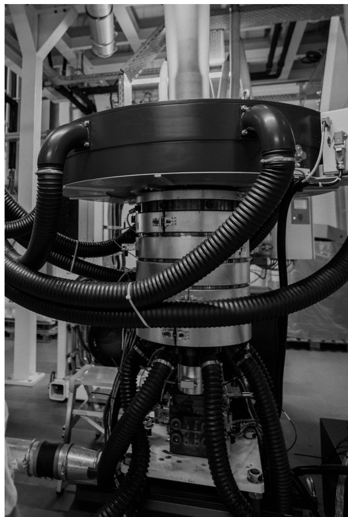
HDPE Long-neck production with Automatic Air-Ring gives maximum performance with automatic and optimum profile improvement
