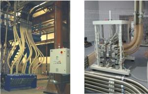
To avoid operator mistakes on material selection the manual solution can be updated with a decoding system, but the safer solution is installing an **automatic material selection manifold**.
