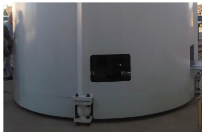
Silo Mounted on Load Cells
