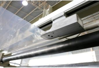
Non-Contact Double Capacitive Layflat Measurement Sensor
