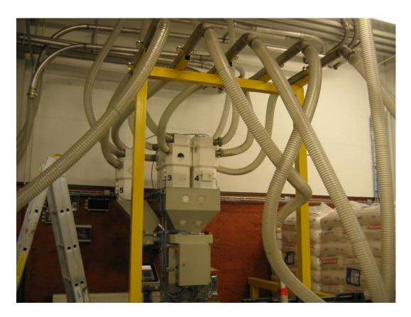
Materials are Loaded into the Blender Reservoir Hoppers from Storage Silos or day bins Beside the System
