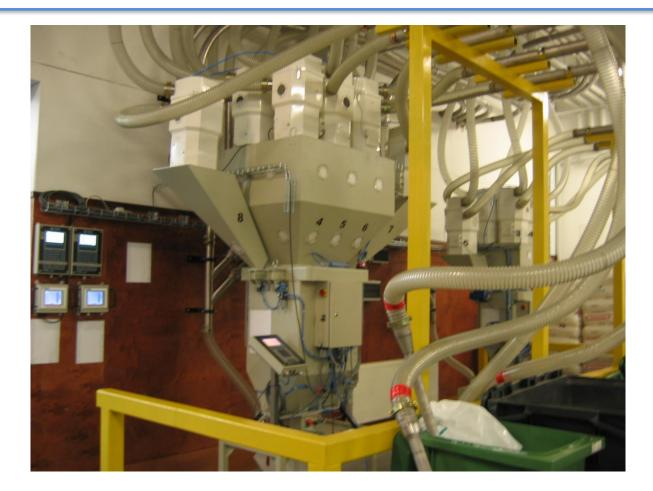
When an Extruder Requires Material, a signal is Sent to the Blender which Prepares and Mixes the Recipe.
