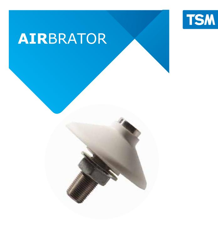
**AIRBRATORS** combines aeration and vibration to solve even the most difficult material flow applications. The special design creates a vibration as the air flows between the pad's boot and bin wall. This provides a very effective flow aid for all types of dry products. Plus, Airbrator pads do not require a specific air pressure for operation. You may use air from as low as 5 PSIG to high-pressure air up to 60 PSIG.
