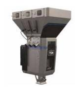
TSM's OPTIX range of extrusion control blenderscombine, in a unique way, accurate gravimetric batch blending togetherwith integrated extrusion control using Loss-in-Weight principle. This results in exceptional ultra fast throughput measurement and control of the extrusion process. The OPTIX range can handle throughputs up to 800kg/hr (1,760lb/hr) and a maximum of 8 components of varying bulk densities.
