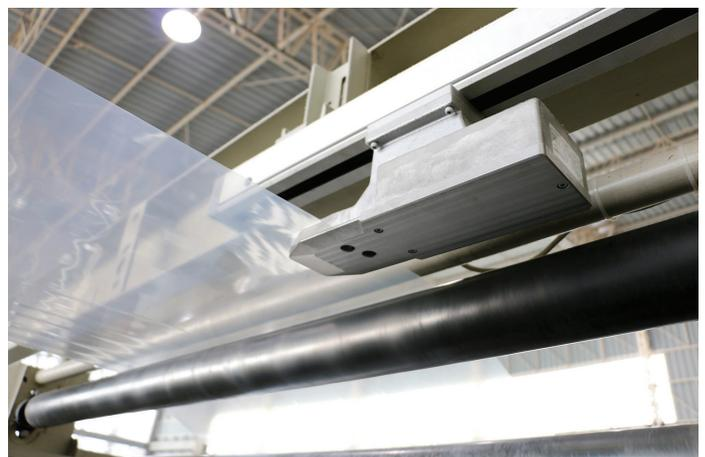
Non-Contact Double Capacitive Layflat Measurement Sensor
